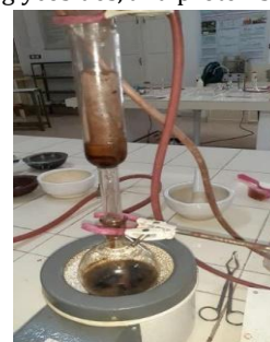
Figure-2: Extraction of embelin
